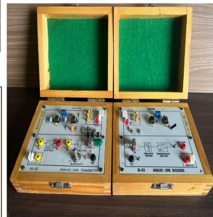
850 nm LED and PIN Photo Diode Module Fiber Optic Analog Link
