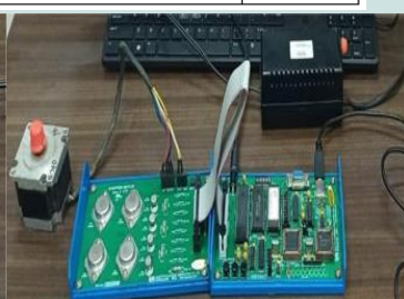
Stepper motor interface with MCB-51
