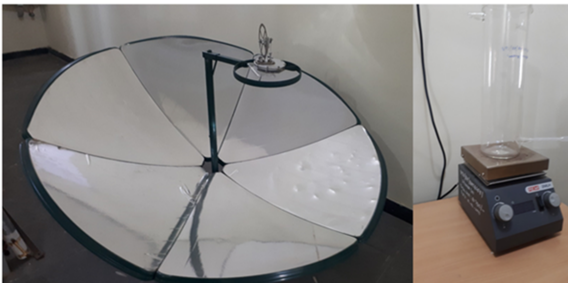
Prototype Stirling engine mounted on the aperture of parabolic dish (left) and fluid analysis setup for convective heat transfer estimation (right)
