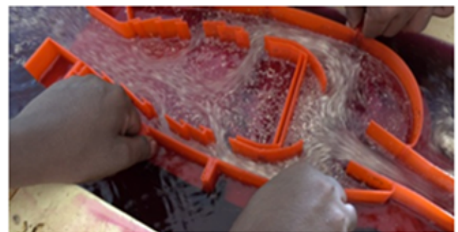
2D Water Tunnel Testing with a Rapid Prototyped Model
